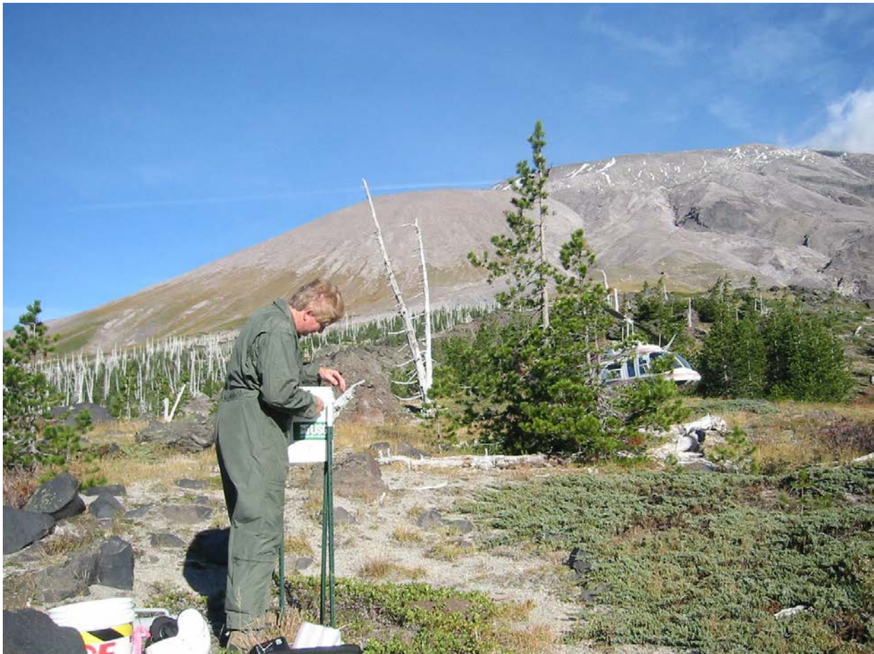
Photograph showing a typical Ash Collection Bucket system used on Mt. St. Helens during the 2004 to 2008 eruptive activity.
