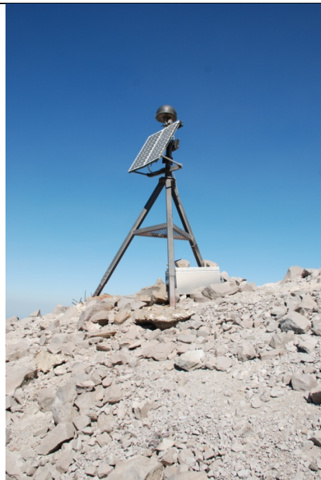
Photograph of an existing Permanent GPS Station located on Mt. St. Helens.
