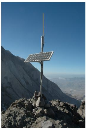
Photograph of a tiltmeter location noting the 2" pole that the solar panel and Omni-directional antenna are mounted on. Tiltmeter buried in ground and the PVC cap is buried under a rock pile to minimize site visibility.
